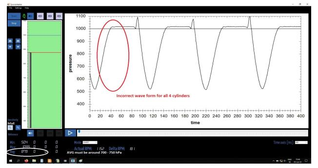
NOTE: AVG too high 879 hPa, its means engine need so much air for idle speed. normally 700-750 hPa
