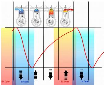
If the engine has a long intake port the diagram will be flattened.
