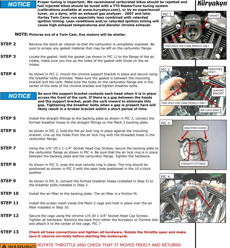
WARNING TO CLOSED BEFORE STARTING BIKE. FAILURE OF THE THROTTLE TO RETURN COULD RESULT IN LOSS OF CONTROL CAUSING SERIOUS INJURY OR DEATH.
